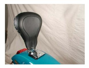
The Harley-Davidson® Chrome Luggage Rack 53806-oo comes with two 3/8"- $16 \times 1\frac{1}{4}"$  bolts and lock nuts, and will mount with the Mustang sissy bar pad. The top bolt provided with the pad is used. To install with the luggage rack, the material must be punched for the second bolt.
