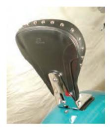
The lower bolt can be installed with the acorn nut on the front or the back as desired.
